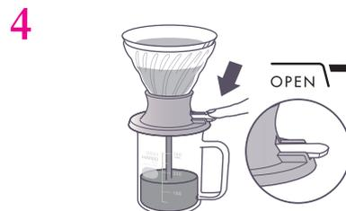
Press the switch to drip coffee. ※Once you have pressed the switch, it will stay released even when you remove your finger. ※A mug can be used in place of a server. ※Make sure to reset the switch before the next time you use the dripper.
